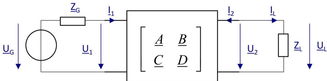
$$\text{Avec } \underline{A} = \left. \frac{U_1}{U_2} \right|_{I_2=0} \quad \underline{B} = - \left. \frac{U_1}{I_2} \right|_{U_2=0} \quad \underline{C} = \left. \frac{I_1}{U_2} \right|_{I_2=0} \quad \underline{D} = - \left. \frac{I_1}{I_2} \right|_{U_2=0}$$
