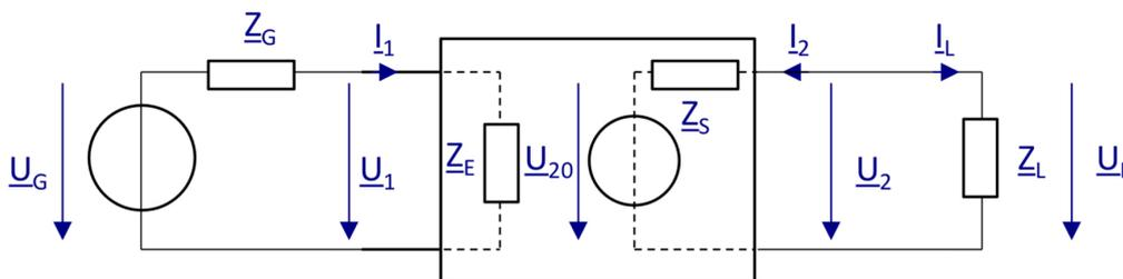
$$\underline{Z}_E = \frac{\underline{U}_1}{\underline{I}_1} = \underline{Z}_{11} - \frac{\underline{Z}_{12}\underline{Z}_{21}}{\underline{Z}_{22} + \underline{Z}_L} \quad \underline{Z}_S = \frac{\underline{U}_2}{\underline{I}_2} = \underline{Z}_{22} - \frac{\underline{Z}_{12}\underline{Z}_{21}}{\underline{Z}_{12} + \underline{Z}_G} \quad \underline{U}_{2,0} = \frac{\underline{Z}_{21}}{\underline{Z}_{11} + \underline{Z}_G} \underline{U}_G$$
